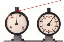
Set pointer to the dot on left dial at start with no load then start applying load
